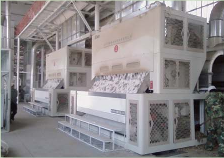
锯齿轧花成套设备系列 Series of Complete Set of Saw Ginning Equipments
