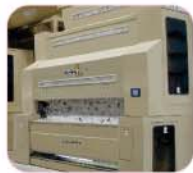
BAJAJ-CONEAGLE 9120 FEEDER & 201 SAW GIN
